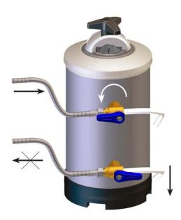
Put the softener back into service by turning the water outlet pipe to the left side.
